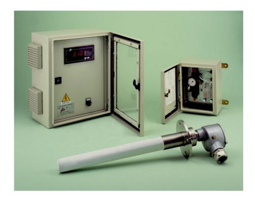
This analyser has the unique characteristic that enables the use in process with extremely wide limit of temperature. (from 100 to 1400°C) It can be used in processes with high particulate content and aggressive atmosphere, like the combustion and post-combustion chambers of domestic and industrial incinerators and all other applications where without extraction or circulation of the flue gas a fast and accurate O2 measure is requested.
