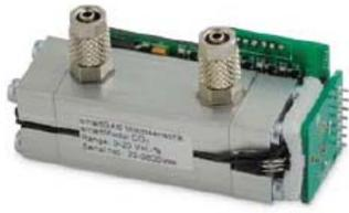
Infrared gas sensor using dual beam technology with measurement and reference channel for use in analytical devices and process control applications. Integrated evaluation electronics for drift and temperature compensation. Robust aluminium cuvette with gas line connectors.
